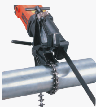
Chain Vise side of the optional 2-in-1 Vise for larger diameters.
