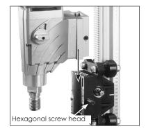
Carefully measure the distance from the center of the intended cut to the location of the mounting slot in the base. Follow the concrete anchor
